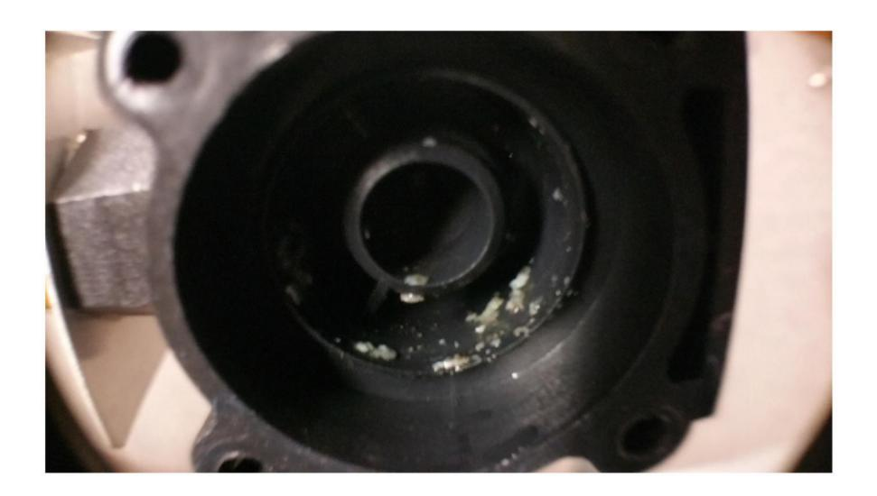
Flush debris from all internal valve parts.
